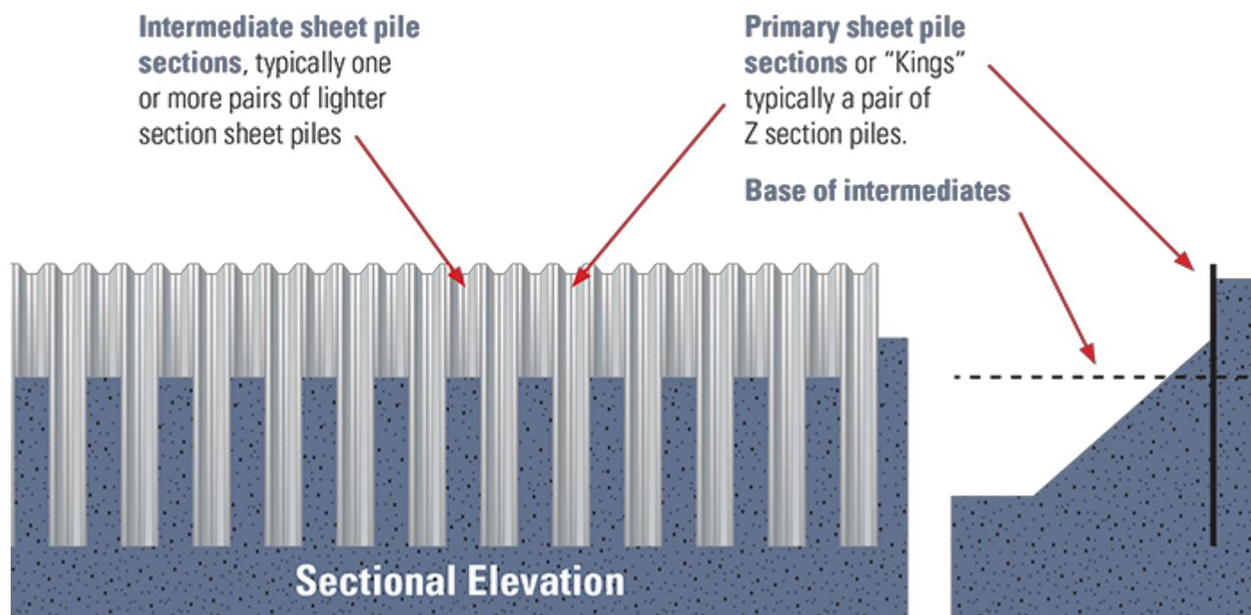
KSP walls are normally designed for use with Z piles. U piles do not work efficiently in a non-continuous wall.
